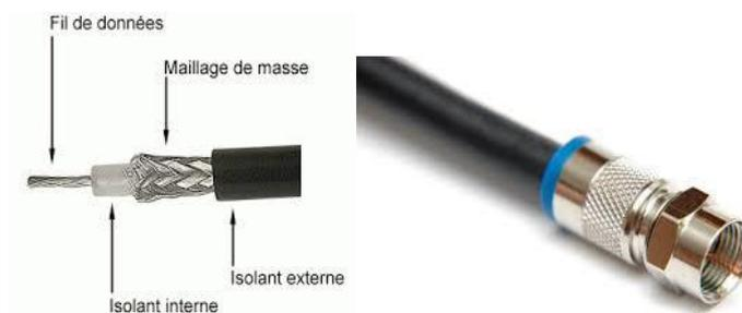
**Figure 1.06 :** *Câble coaxial*
