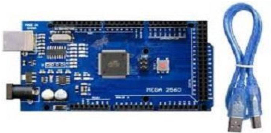
**Figure 3.01** : Arduino MEGA [1.14].
